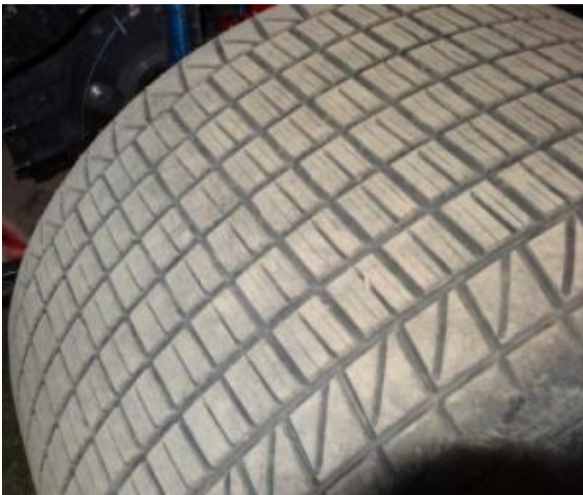
Right rear after a full night and 30 lap feature on a \frac{3}{8} mile track
