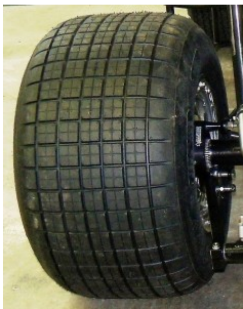
The SOD left rear is a Hoosier 92/12.5-15, D15 compound.
