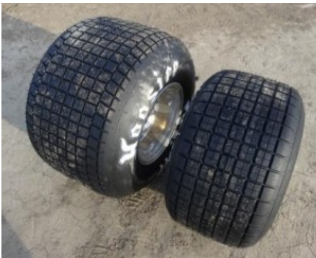
2016 SOD spec tires. 100/13-15 medium and 92/12.5-15 D15
