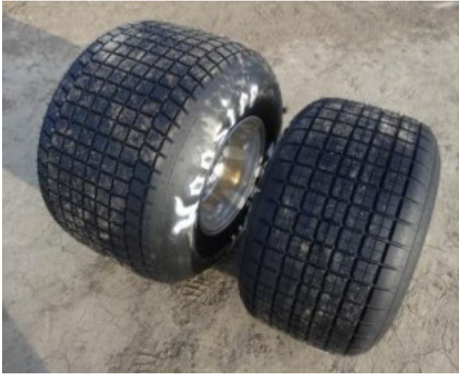
2016 SOD spec tires. 100/13-15 medium and 92/12.5-15 D15
